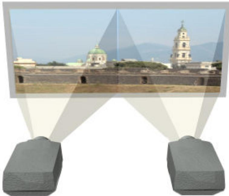
In this configuration, each picture is lined up to its neighbour exactly along a common edge. In Delta, Set Channel 1 & 2 to exactly half of the canvas size, and set Channel 2 to have an X Offset of half the canvas size. No blending is required for this system.
