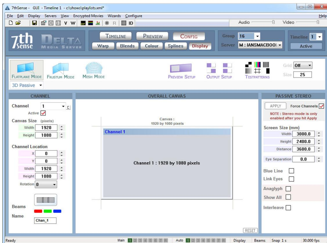
In this mode, the canvas is divided into 2 channels, one for left eye and one for right eye. Each channel is output through a separate video output to a projector, which are exactly overlaid on the screen, each projector having a different polarisation. Using inexpensive passive stereo glasses, each eye receives only the polarised image for the relevant eye, and in this way, each eye sees a slightly different view, creating the stereo depth.
