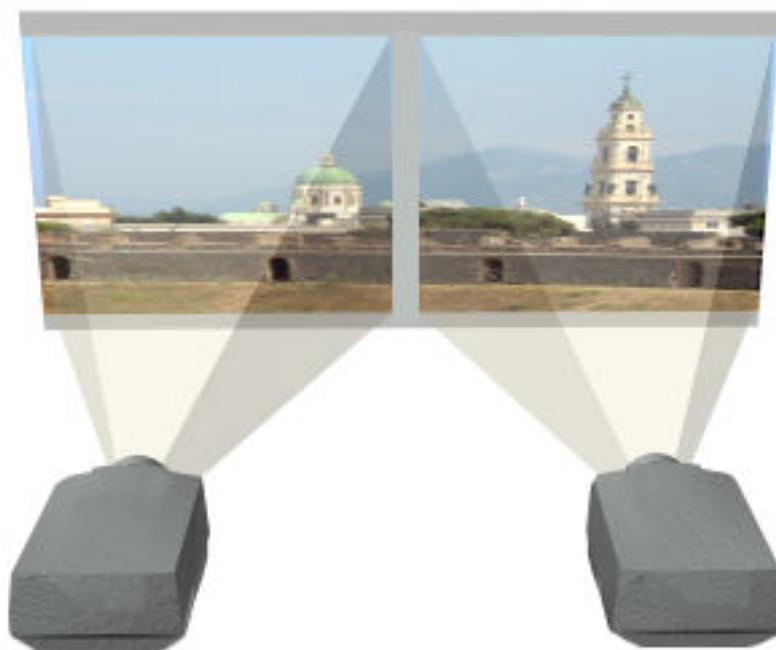
In this display, the projected images have a physical gap, so the Delta imagery must also have a gap otherwise things will not “disappear” properly in the gap.
