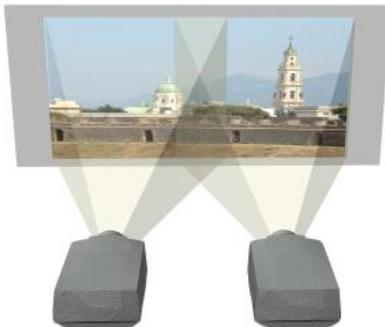
In this display, the projected images are physically overlapped (usually by 10%), then a blend is applied to the left and right edges to provide a seamless display.
