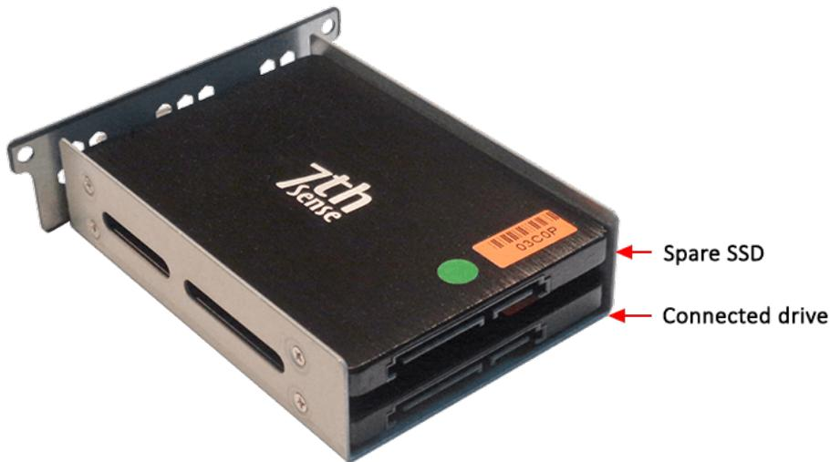
The SSDs are each held in place by four small screws. The upper disk is the spare (factory clone), and the lower is the C:\ drive.
