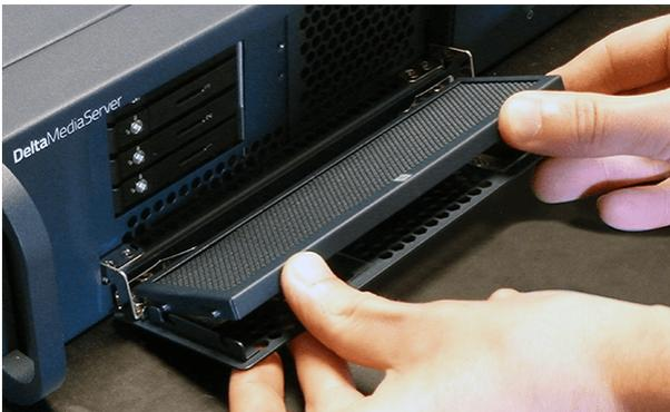
Pull down the filter door, and push the carrier forward evenly against the spring clips. Note the orientation of the carrier with the magnetic catch spot at the top.
