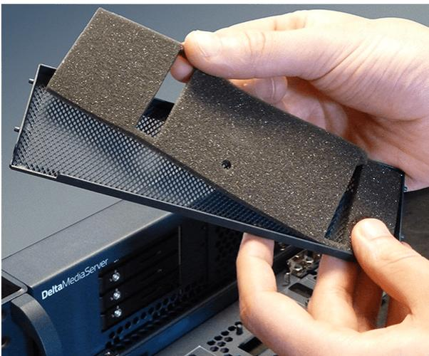
Remove, clean or replace the foam, noting the orientation of the cutouts.
