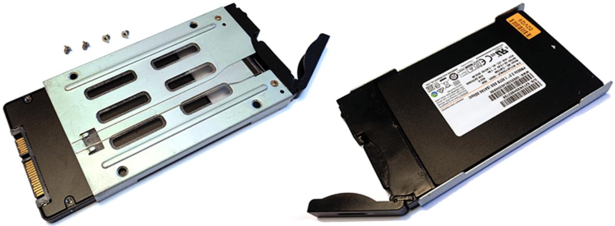
Replacement is the reverse process. Ensure that the new drive is locked and the retaining bar screwed back in place.
