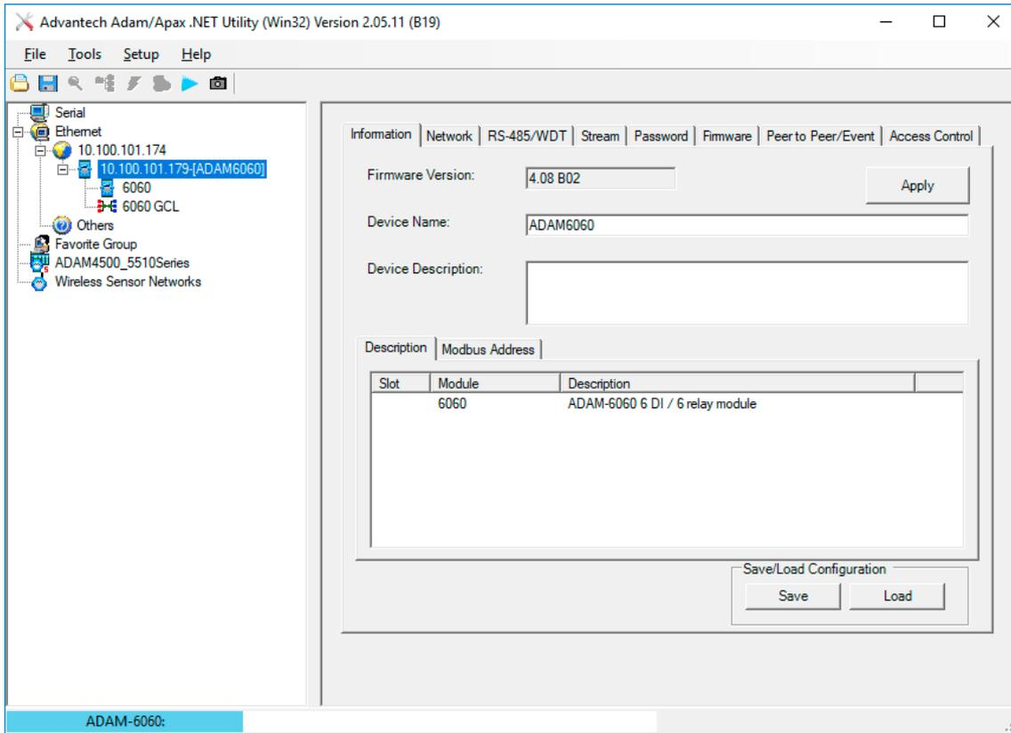
Select the **Network** tab and note or change the ADAM-6060 IP address as required (example: 10.100.101.179). The ADAM-6060 must be on the same subnet range as the Delta server.
