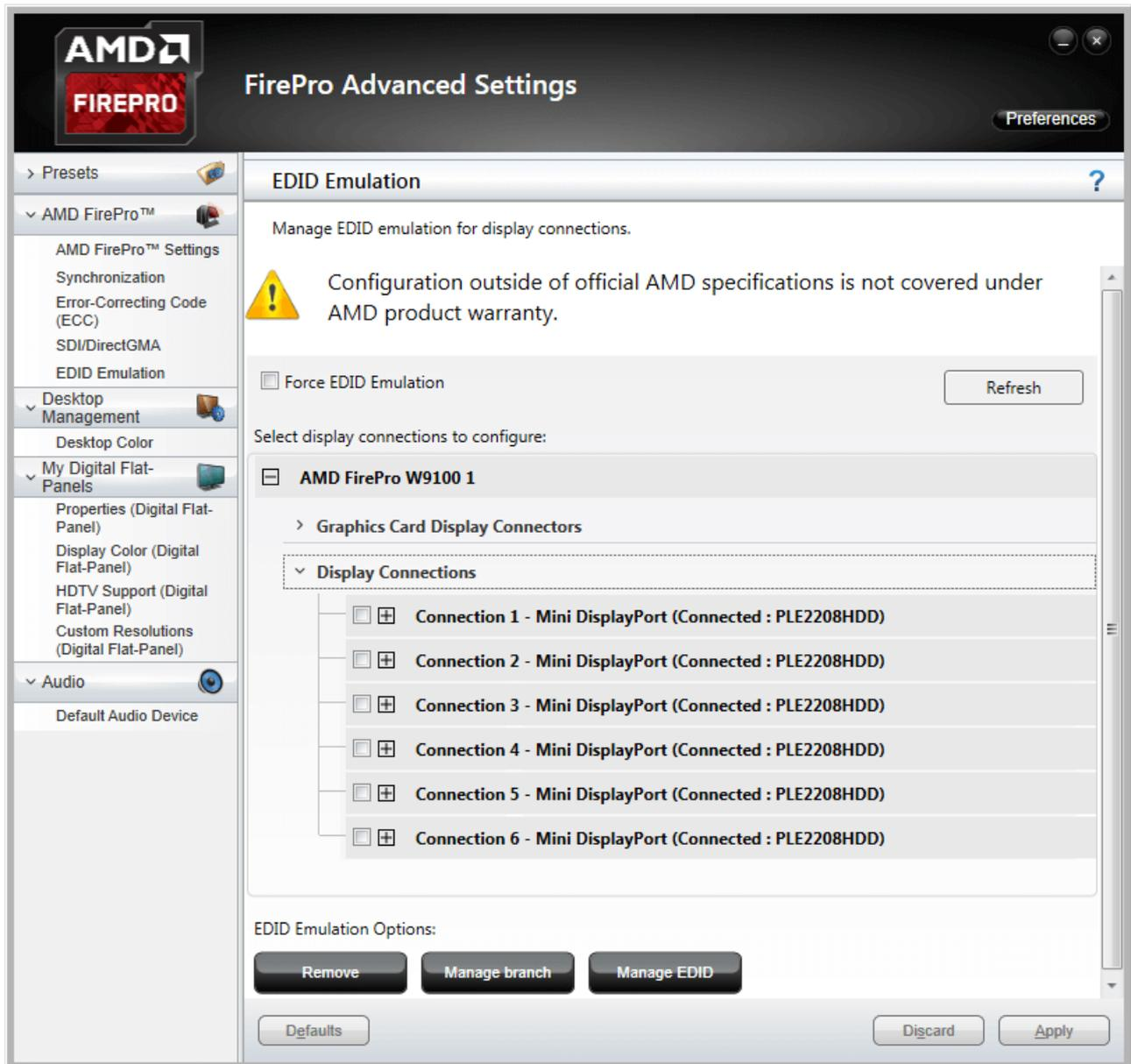
On this GPU, there are 6 available ports, showing what type of connections there are. In this instance, the GPU supports Mini DisplayPort
