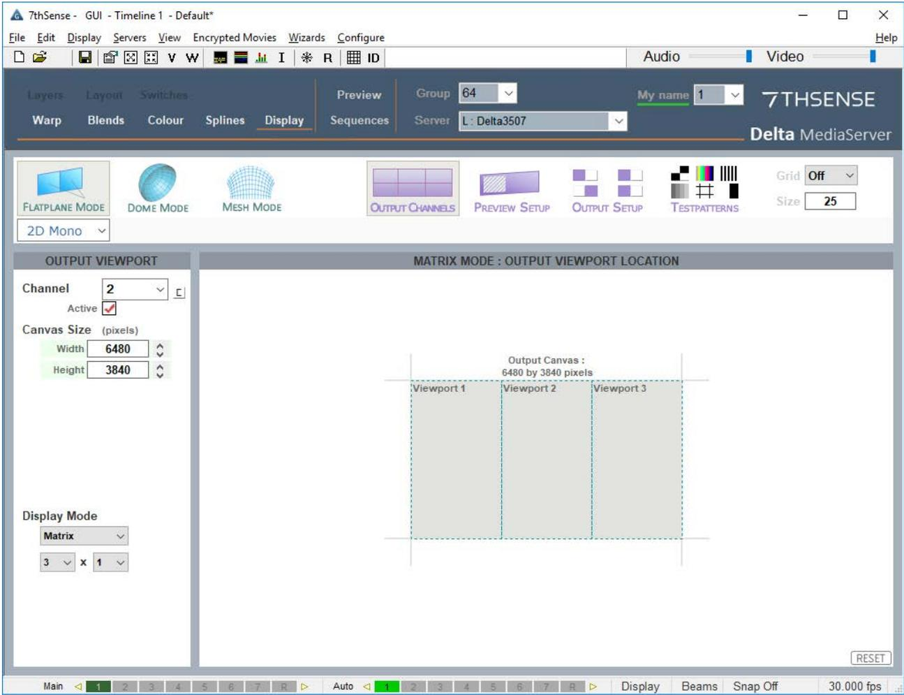
The three **channels** are rotated to match the graphics card grouping for portrait-oriented displays, so that they run left to right:
