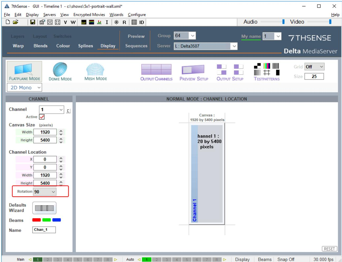
The **media** is in the correct physical orientation for the display and therefore agrees with the channel, not the canvas, so we give it a corrected location in the layout. This is easiest by positioning the centre of the media in the centre of the canvas:
