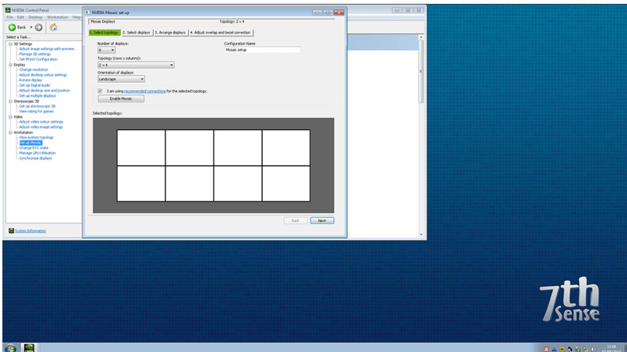
Along the left-hand side, select *Set up Mosaic*. Select the number of outputs you wish to use, and then the arrangement you need. Click the tick box 'I am using recommended connections for the selected topology' and then click Next.
