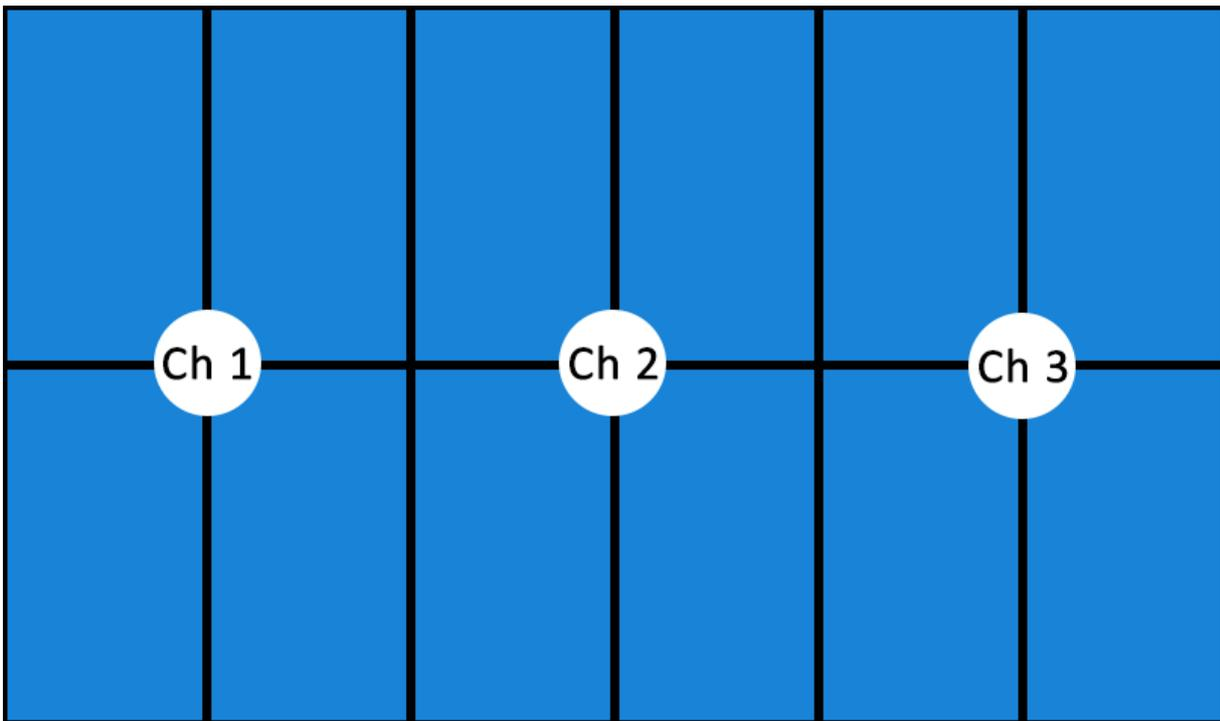
In DeltaGUI, the **canvas** matches the overall display, in an underlapped (for bezel compensation)  $3 \times 1$  matrix array:
