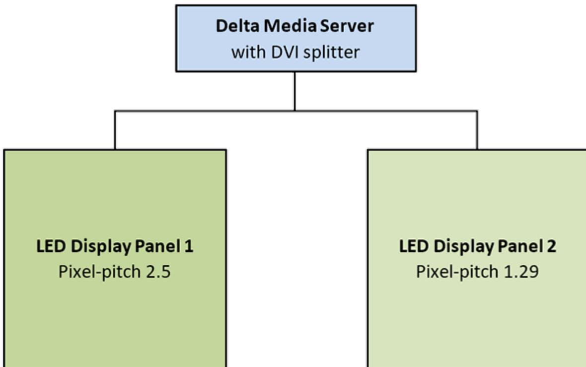
By using DeltaServer in [composition mode](#) (a Delta licence option), the output channels can be manually placed on the output raster. Each LED processor receives only the relevant part of the media, on a desktop resolution in DeltaGUI that matches that of the processors.
