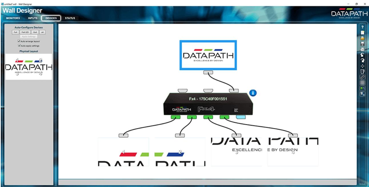
Any element can be clicked to show its properties, and/or dragged: selected items go green. You can reassign outputs to panels by dragging the wires. This avoids the need to swap plugs and ports to correct physical arrangements.
