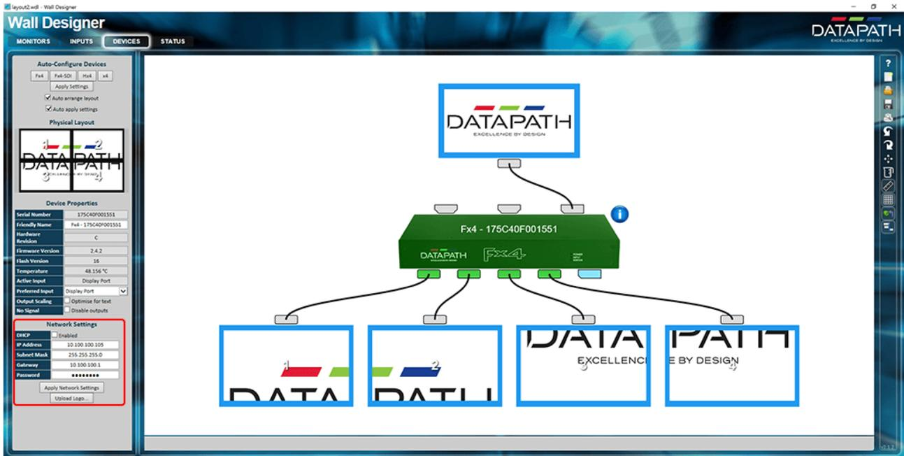
You can now set a static IP address for using the remote browser Wall Designer app to log into the Fx4 unit. Apply (and note) a password. This will be required at the Fx4 IP Control Panel when you try to connect to the IP of the Fx4.
