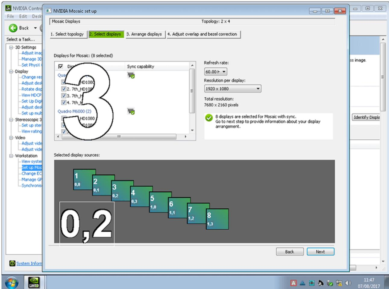
In the next stage, you can re check that the desired Refresh rate and Resolution will be set for each display. Each connected display will show with a number in the foreground for reference.
