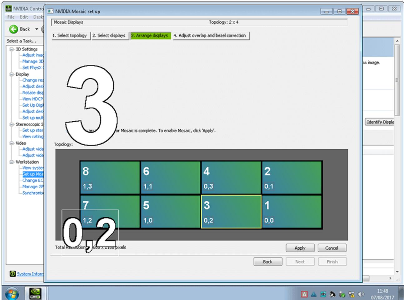
You will then need to drag the corresponding screen number on the top to the arrangement below to make sure the outputs are in the correct displayed order.
