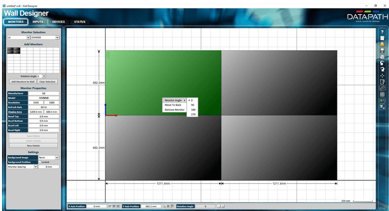
Here one monitor has been selected (just click and it will go green, showing the origin point), and the right-click menu shows rotation and layer, and allows removal from the wall. The measurement tool has been applied: click this tool once for overall dimensions, again for panel dimensions. Units can be mm or in, using the 'toggle units' tool.
