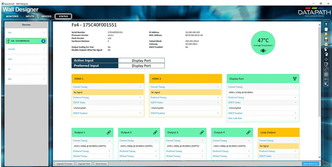
The Status Panel provides a detailed summary of the device including details of Flash and Firmware versions, IP Address (if connected via a network), serial number and average temperature of the device etc. The Status Panel also displays the input and output properties. A detailed view of each property can be viewed by clicking on each drop-down menu.
