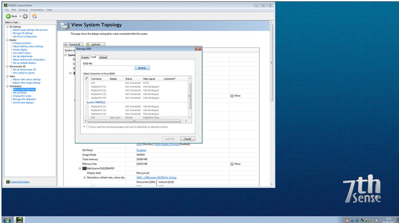
This will then open the **Manage EDID** window. Ideally when spoofing EDIDs, you want to use the native display EDID file. 7thSense do provide a wide library of common EDID files on the server, though these should be used only if necessary.
