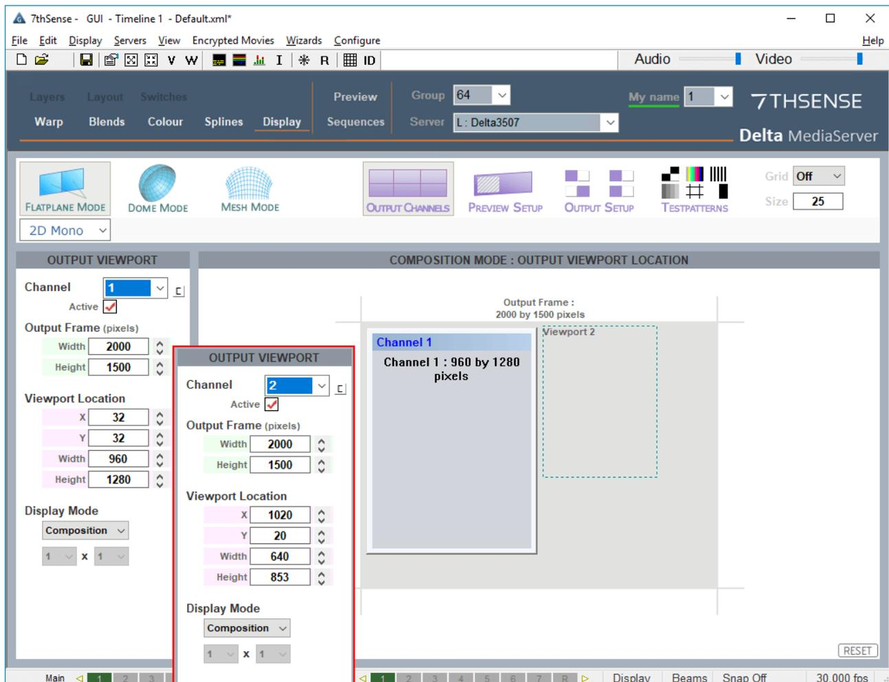
**Channel 1 viewport** location has been offset in X and Y by 32 px (let's say this is a requirement of this LED display panel). Its width is the first (horizontal) half of the media (960), and it is full height (1280).
