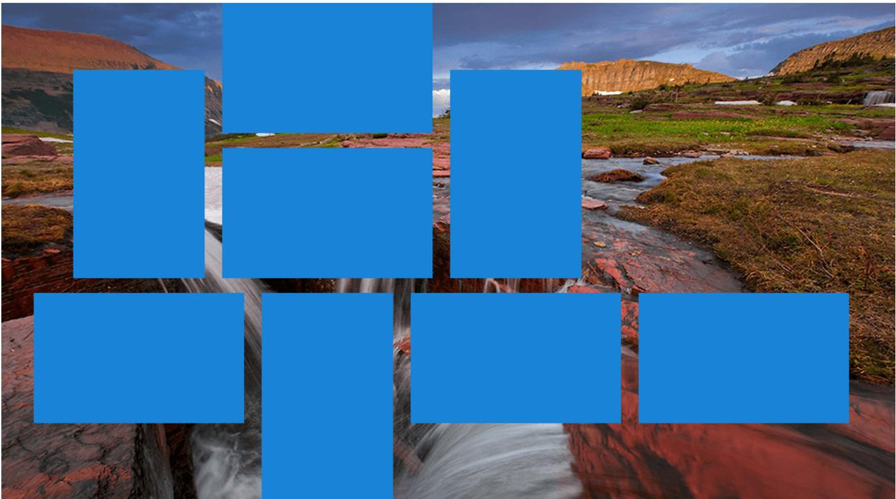
Delta software offers [composition mode](#), whereby elements of the source media are placed individually into display areas. This allows for very efficient media delivery by compacting just the visible areas during the graphic design, into a rectangular frame that minimises unused pixels.
