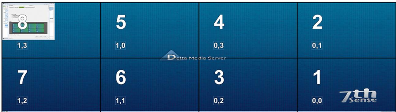
The outputs will then flash for up to 1 minute while the Mosaic is set up. When this is complete, double check all outputs are in the correct place. Once complete, click Finish. If bezel compensation is offered ignore it, it is advised that this is corrected for in the Delta canvas, rather than in the graphics driver. Once mosaic is complete, please restart the Delta server.
