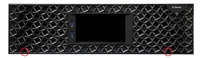
After removing the two screws, pull the fascia forwards and straight off the unit. It is retained by four push-fit fasteners. Refit the fascia after mounting. Where side access is restricted for unracking, a 7thSense tool is available to insert into the grille. Take care not to damage the grille with other tools, or force when removing.
