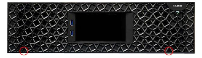
After removing the two screws, pull the fascia forwards and straight off the unit. It is retained by four push-fit fasteners. If the fascia sides are inaccessible, plastic hooks are provided to pull the fascia off (see <a href="Installation">Installation</a>.
