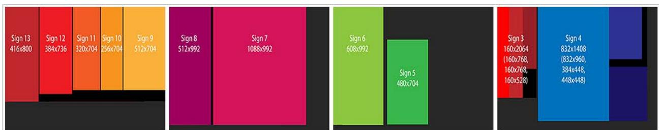
All we need to do now is to find the coordinates and dimensions of each LED panel in the packed artwork, make each a channel, and then place the viewport for each channel in the output, according to this plan.
