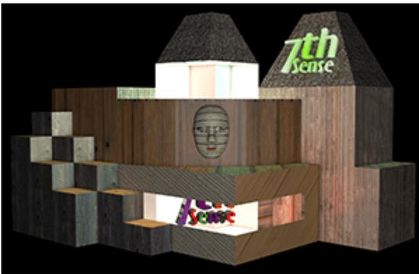
Because the designer's reference point is the origin of the model, the media effectively represents what the origin of the model would see in a mirror. For better and sharper results, the media can be displayed over several projectors, and it may be better to split a complex mesh model into more manageable pieces for those projectors, but projection mode still assumes that the designer and viewer are both looking at the media-painted object from the same view of the model.
