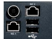
On the rear right-hand side, the RJ45 port labelled 'NIC 1' is factory-set to a static IP and 'NIC 2' to DHCP. A label with this initial static IP address is provided on each unit.
