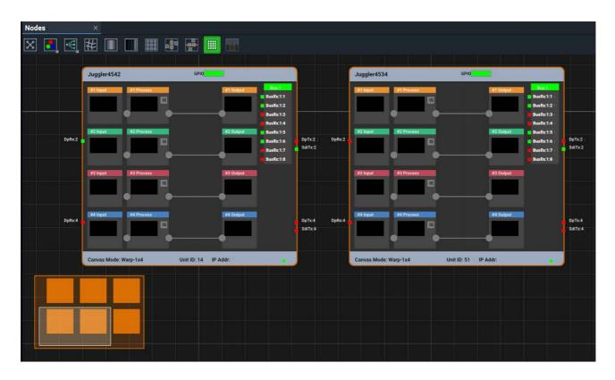
The orange box contains all objects. The lighter area is the current view scope and can be dragged around to view the required Juggler(s) without having to zoom out or in to find your bearings.
