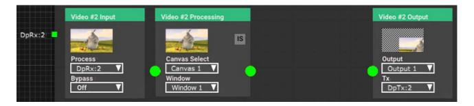
Now we have NDI showing an input signal is being received, that it is being presented to a named window, and where it is being displayed on the named output.
