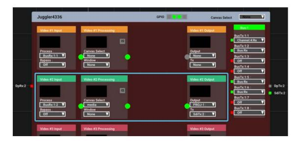
The square pins on the left and right margins represent the physical input and output connectors. When a signal is present they are green, and when disconnected they are red.
