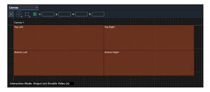
A similar output canvas mode is available to 4-lane bus systems, but instead of each video channel connecting to two bus lanes, they each connect to one. In effect this is as above, but with only a single output. By applying a further 'dual stream' mode, this also can be split into two outputs.
