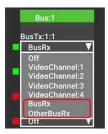
'BusRx' refers to the channels placed on the local bus, and the 'OtherBusRx' refers to the channels from the second bus. This switch would reassign the backup channels to the bus, in place of the primary channels. After this switch, within each juggler that is supporting a physical output, the processing channel is selected from the bus that is now carrying the corresponding backup input channel.
