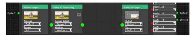
On the left is the square green Juggler module input pin, here DisplayPort #2 (DpRx: 2). It is showing green because a valid media feed has been detected on it.
