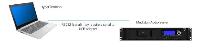
Connect an RS232 cross cable to the COM 1 port on the rear of MAS Pro Dante DH and use HyperTerminal for external commands.
